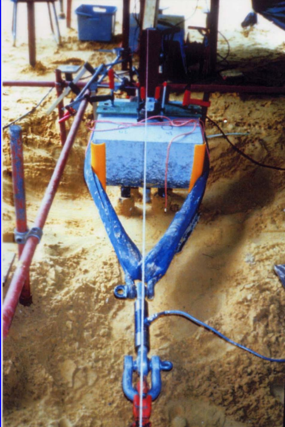
Horizontal loading test of
